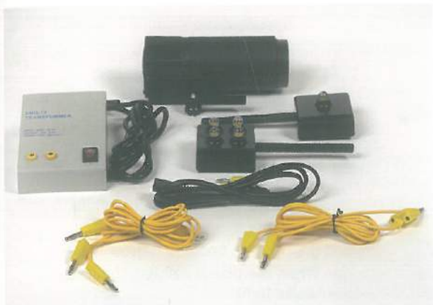
Projector with transformer, cables and lamp holders.
