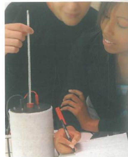
Joule's Law Unit setup with the Calorimeter.
