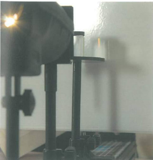
Detail of the equilateral prism mounted on the optical bench.
