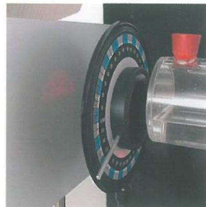
The angle is adjusted until all light is blocked out.
