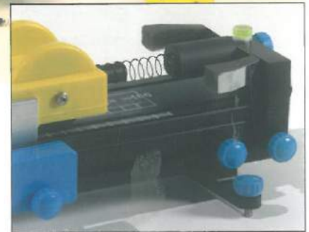
Detail of the elastic collision between cart and bumper.
