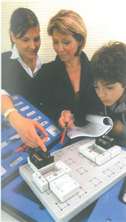
Series and parallel sample circuits experimental setup.
