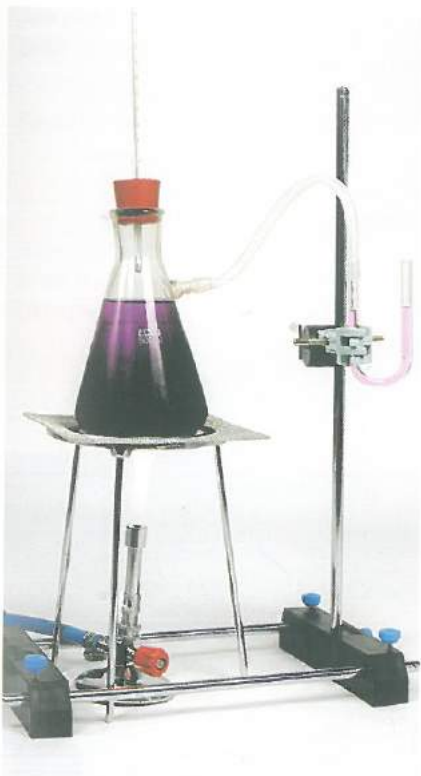
Detail of the air expansion in the U-Tube manometer.
