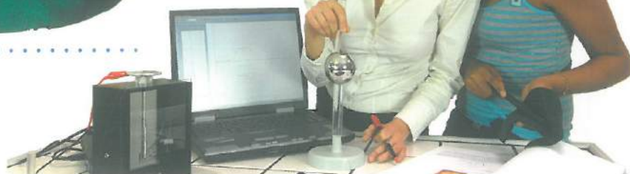
Measuring charge in a hollow sphere with electroscope and datalogger.
