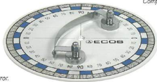
A biconvex lens placed on the Hartl disk.
