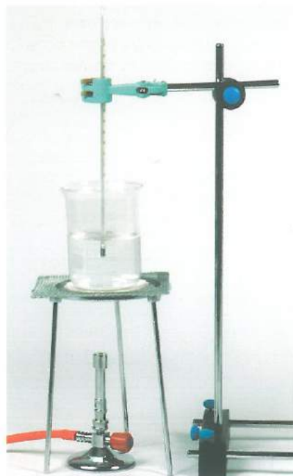
With just a beaker, boiling water and a thermometer it is possible to measure thermal sensitivity.
